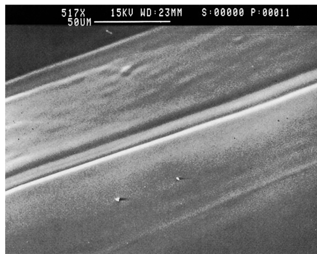
Figure 11 Dependence of the morphology of the coatings on the weight gain of fibers (top = 27.9 wt %; bottom = 54.5 wt %).
